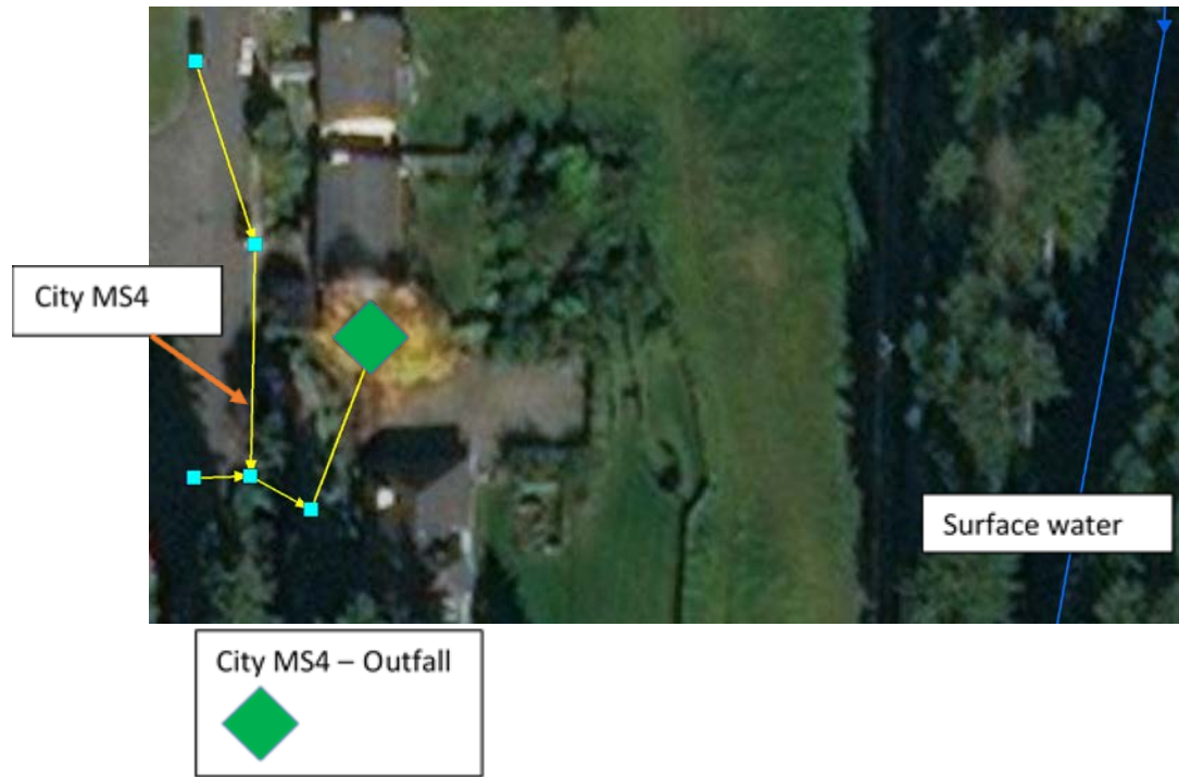
Figure 8. In this scenario, the City maps the location where discharge leaves the MS4 as an outfall because the City has knowledge the discharge will enter a surface receiving water.
