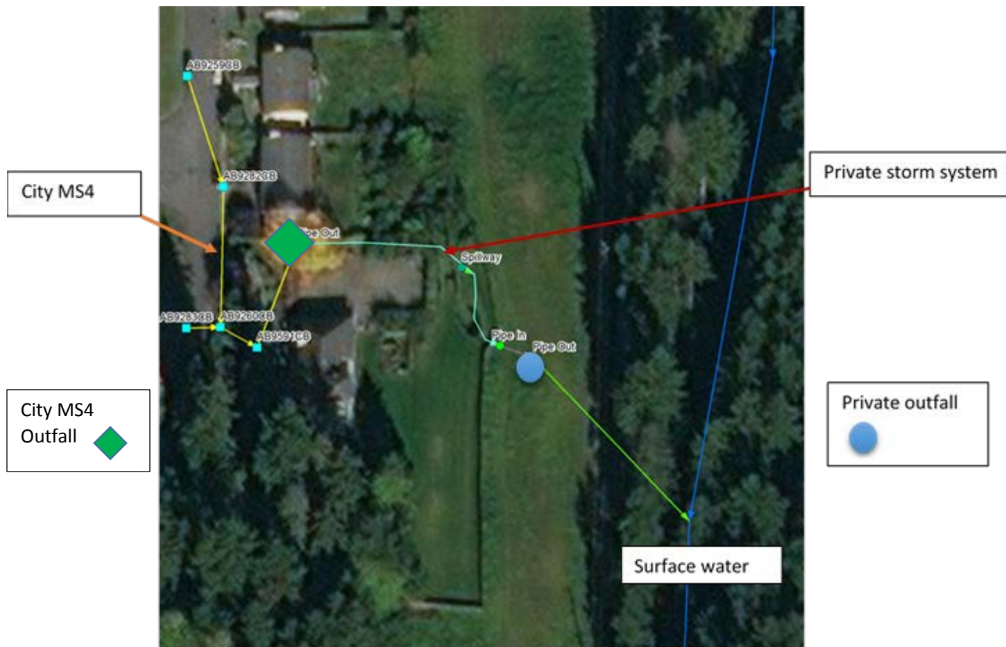
Figure 7. Municipal system to private stormwater system.
