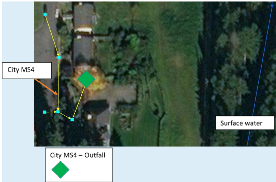
Figure 8. In this scenario, the City maps the location where discharge leaves the MS4 as an outfall connection point because the City has knowledge the discharge will enter a surface receiving water.
