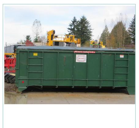
Photo 2 – Dumpster lacking stormproof lid. Lid has cracks between the plates that allow precipitation to seep in (Photo 3). Dumpster needs to be turned around so water sheds off. Metal shavings noted on ground around dumpster (Photo 4). Dumpster has been changed out for one with storm proof lid by July 27 inspection (see photo 11).
