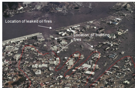
Fig. 17. Combustible material beds surrounded with red line in a harbor district on 12th March 2011, The rightmost area caught fire on 14th March 2011 by unknown process (Kesennuma city, Miyagi prefecture) [21].
