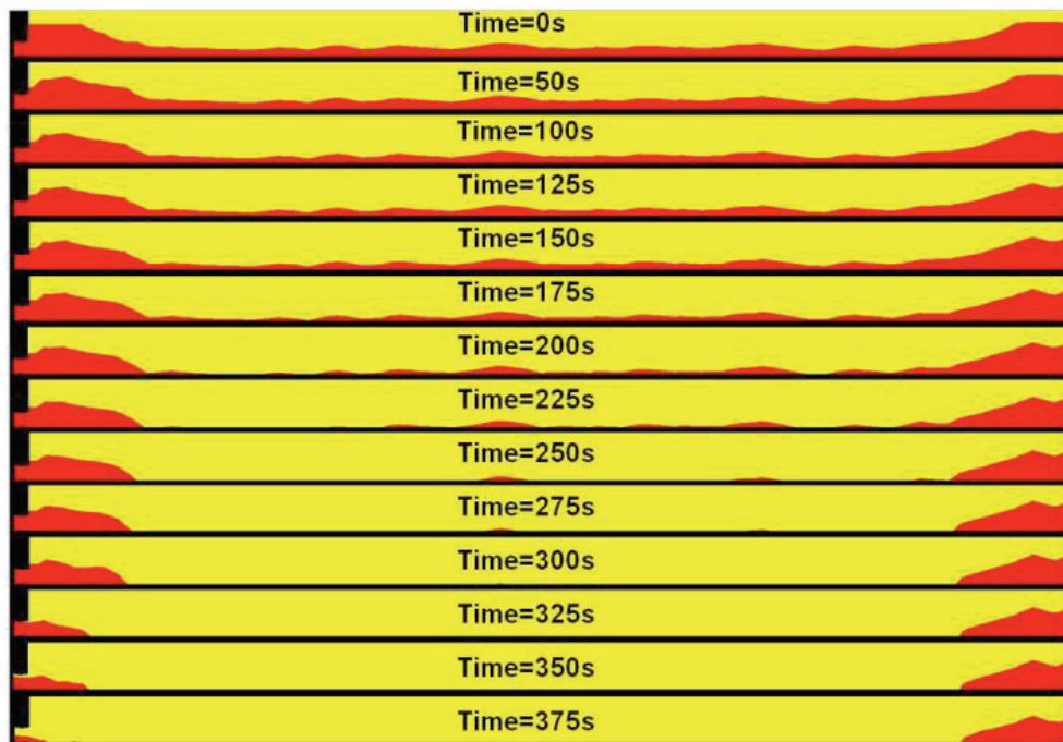
Figure 5. The ferrosilicon level during the tapping process. The gas phase is represented as yellow. The ferrosilicon (shown in red) is forced to the furnace periphery due to the static gas pressure in the furnace
