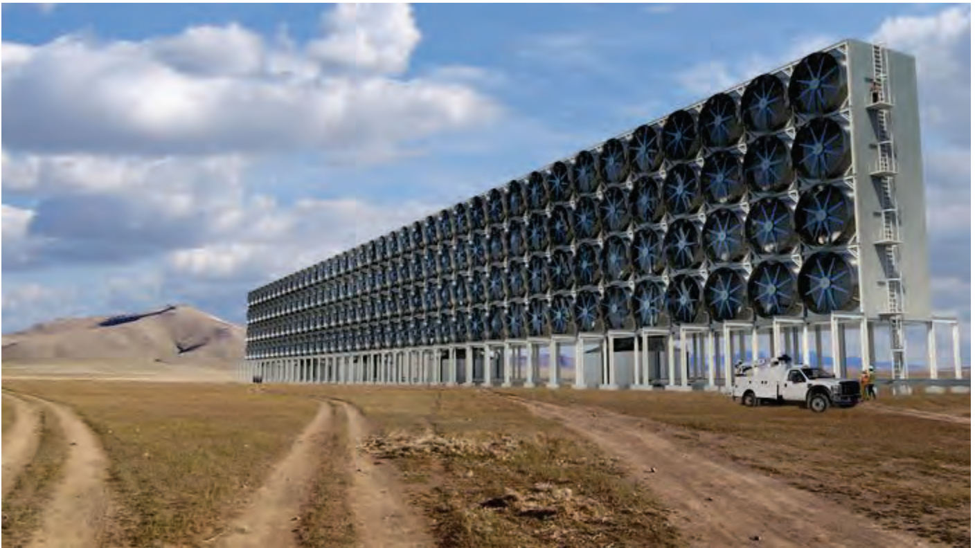
Air-contactor assemblies remove carbon dioxide from the atmosphere. (Carbon Engineering via AP)
