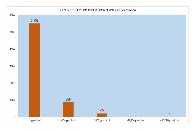
As shown in the above graph, 222 data points had methane concentration above 500 ppm, and 3 data points were above 50,000 ppm. The highest methane reading was at 82,400 ppm, these are a significant emission of raw LFG into the ambient air!
