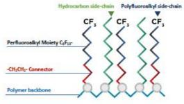
Composition and Structure: Side-Chain Fluorinated Polymers are a hydrocarbon polymer backbone with a polyfluoroalkyl side-chain bound to the backbone that contains a six-carbon perfluoroalkyl moiety as well as side-chains that have no fluorinated carbons.
