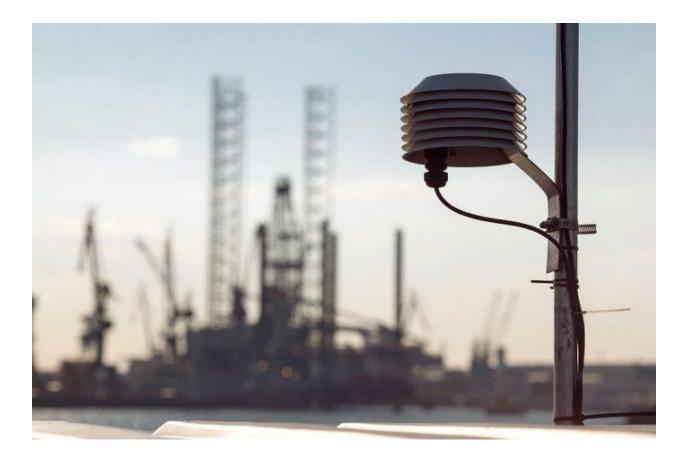
Some substances are toxic, dangerous, or unpleasant. The sensors in the E-nose and resonator sensors take measurements of odorous and odorless gas compounds in the vicinity. The measured gas compound is compared with the chemical fingerprints of known compounds recorded in a central cloud database.
