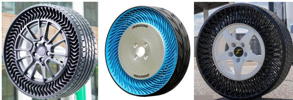
Figure 4.1 Examples of Non Pneumatic Tire Products. Sources (left to right): Michelin, 2023; Bridgestone Corp., 2013; Goodyear, 2023.
