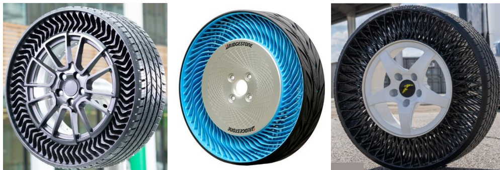
Figure 4.1 Examples of Non Pneumatic Tire Products. Sources (left to right): Michelin, 2023; Bridgestone Corp., 2013; Goodyear, 2023.
