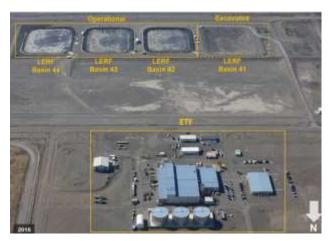
LERF Basin 41was dug out in 1990. Now USDOE proposes to add clay and geotextile liners for a 7.2 million gallon basin. Is this the design that would be chosen if the basin was not already dug out (which was done before USDOE acknowledged that RCRA hazardous waste law permitting applied)? The permit lacks groundwater monitoring provisions.
