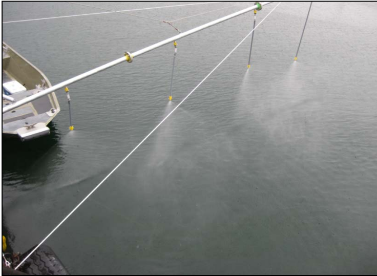
NRC's AylesFerne BoatSpray 100 port side spray arm being tested with water at Neah Bay, WA
