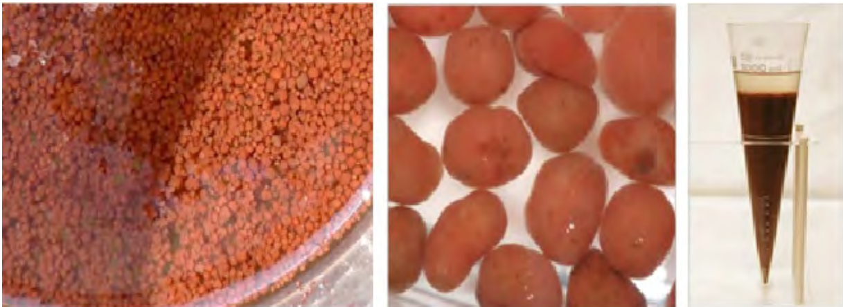
Anammox Granular Biomass
