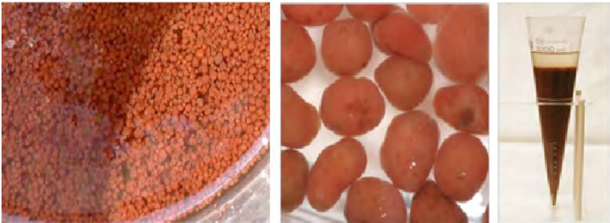
Anammox Granular Biomass
