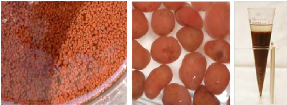
Anammox Granular Biomass
