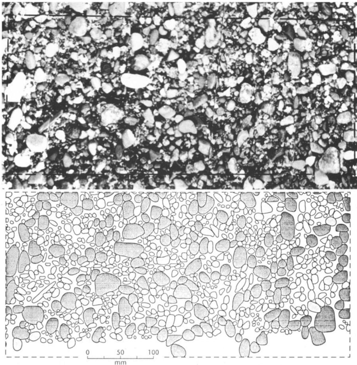
**Figure 3.** Pattern of large stones on the bed surface after the experimental flume run 10-3; the vertical photograph and drawing are to the same scale. The darkly shaded stones are those larger than  $D_{84}$  (12 mm) and the smaller stones in interlocked contact with them that form the reticulate structure of the bed surface. Different analysts operating independently identify the same structural pattern from the photographs.
