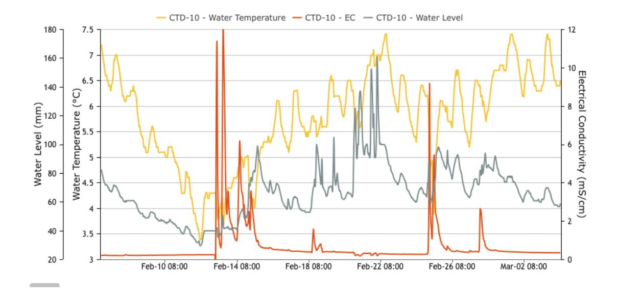
Real time logger at Trib 3A showing conductivity spikes during cold weather in February
