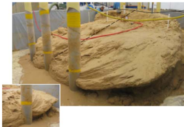
Figure 4. Image of a cemented sand body from a large scale Biogrout experiment. Reprinted from van Paassen et al. (2010), with permission from ASCE.
