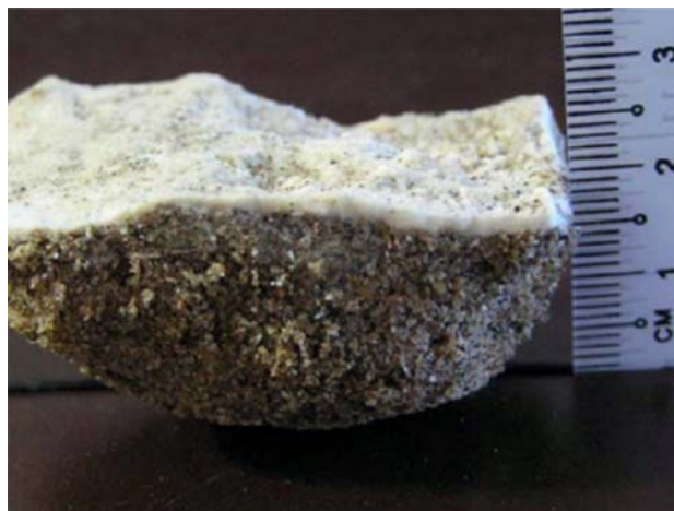
Figure 5. Photograph of an ~1 mm thick crust of calcite on a sand surface. Reprinted from Stabnikov et al. (2011), with permission from Elsevier.
