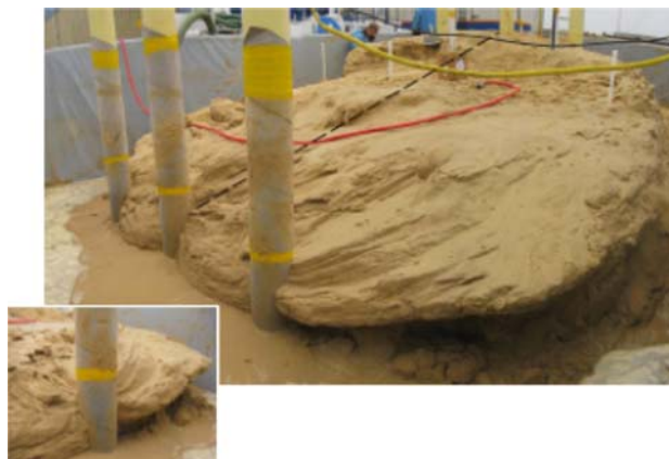
Figure 4. Image of a cemented sand body from a large scale Biogrout experiment. Reprinted from van Paassen et al. (2010), with permission from ASCE.
