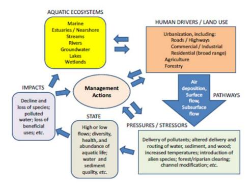
Figure 1: Stormwater Stressors and Pathways
