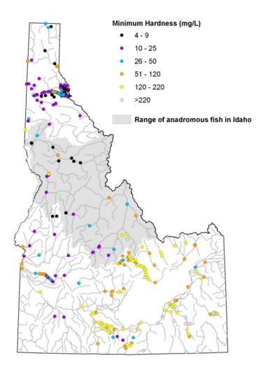
There are, as the figure indicates, many waters in Idaho with hardness levels below IDEQ's proposed hardness floor. Calculating criteria for metals that are hardness dependent using the
