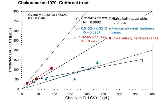
Figure 9. Cutthroat trout modeled and predicted responses to copper under various combinations of low, medium, and high hardness and low, medium, and high alkalinity, in waters with DOC ranging from ~0.9mg/L in low alkalinity water to 3.3 mg/L in their high alkalinity spring water, 2.7 to 9.7g fish (Chakoumakos *et al.* 1979). Because DOC was nearly uniform within alkalinity treatments, data are grouped by alkalinity groups.
