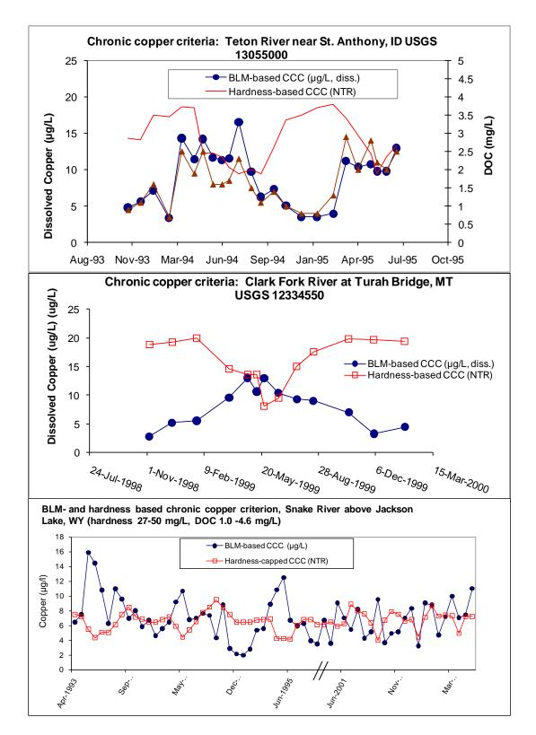
Figure 26. Seasonal patterns in BLM-CCC and hardness-based CCC in streams with a strong spring snowmelt influence, and moderately-hard to softwater chemistry: the Teton River, ID; the Clark Fork River, MT; and the Snake River as it leaves Yellowstone National Park, WY. A consistent asynchronous pattern is apparent where the BLM and hardness-criteria shift in opposition to one another.
