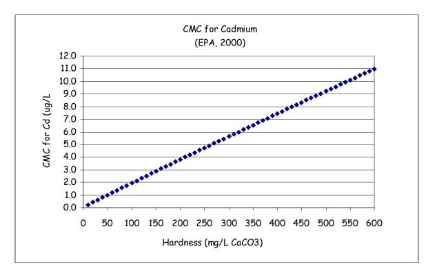
Figure 7. "Quick lookup" graph for the Cd CMC. If water hardness is known, the CMC can be visually estimated. Similar graphs for other metals can easily be constructed.
