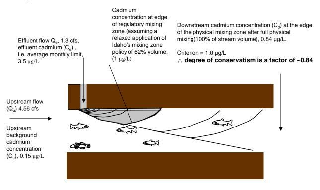
$$C_d = \frac{C_u Q_u + C_e Q_e}{Q_e + Q_u} = C_{\text{(downstream)}} = \frac{(0.15 \,\mu\text{g/L} \cdot 4.56 \,\text{cfs}) + (3.5 \,\mu\text{g/L} \cdot 0.87 \,\text{cfs})}{(0.87 + 4.56) \,\text{cfs}} = 0.84 \,\mu\text{g/L}$$
