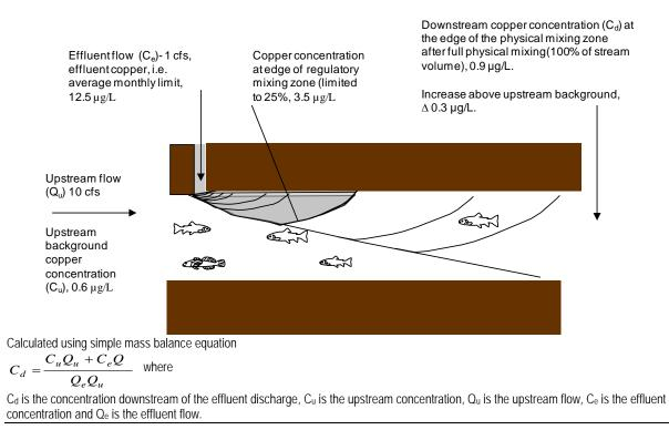
Figure F-2. Illustration of effluent limit calculations and resulting copper concentrations for a springtime, low-hardness scenario where the volume of the receiving water allowed to be used in calculated the effluent limits was limited to 25% of the actual stream volume.
