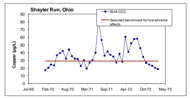
Figure 21. Seasonal patterns in BLM-chronic criterion in Shalyer Run field study, in comparison to an estimated benchmark of adverse effects based on streamside tests. Average hardnesses 180 (126-220), DOC 6 (4-12 mg/L), pH 8,1 (7.75-8.3). Original data from Geckler *et al.* (1976).
