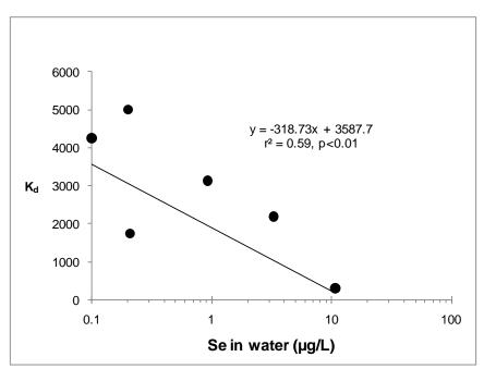
Figure 2.4.8.2. Apparent concentration dependence of selenium water-particulate partitioning coefficients (K<sub>d</sub>) from coldwater, salmonid streams.
