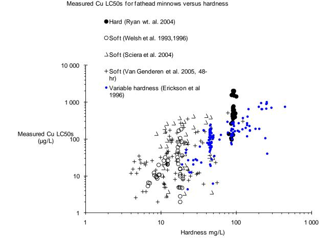
Figure 5. Hardness as a predictor of copper toxicity to fathead minnows: at a hardness of 20 mg/L, fathead minnow LC50s could range from about 2 to 300 µg/L, and at a hardness of about 90 mg/l, LC50s could range from about 100 to over 2000 µg/L.
