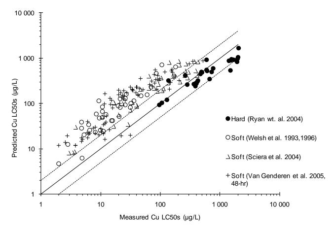
Figure 4. Fathead minnows, BLM predicted and measured Cu LC50s labeled by hard or soft dilution waters, using BLM v 2.2.3 and EPA's 2007 LA50. The comparison shows the BLM generally underpredicted toxicity in the more toxic samples with low measured LC50s.
