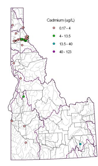
Figure 6a. Cadmium value associated with minimum hardness value (n = 90)
