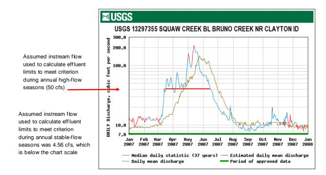
Figure D-2. Examples of actual stream flows versus stream flows that were assumed to calculate seasonally variable wastewater discharge limits for a facility. Actual flows were estimated to be lower than the seasonally adjusted assumed flows about 98% of the time (IDEQ 2000; EPA 2000).
