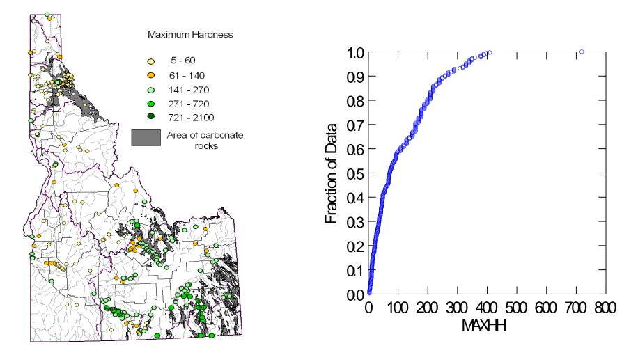
Figure 2. Map showing maximum hardness measured from 1979 to 2004 and areas of carbonate rock in Idaho.
