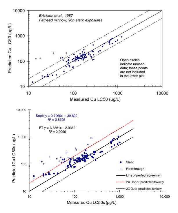
Figure 2. Top - Biotic ligand model predicted versus observed LC50 values for fathead minnows in static toxicity exposures. Figure is from EPA (2003, their Figure 14) in which data from Erickson *et al.* (1987, 1996) were used with the BLM parameters and a fathead minnow LA50 of 6.32 listed in Table 1. The solid line is the 1:1 line of perfect agreement and the dotted lines show the 2:1 and 1:2 lines showing
