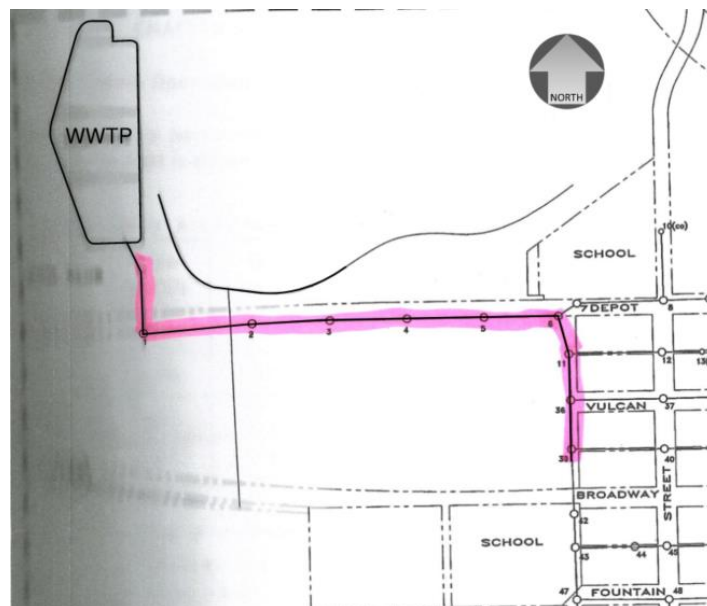
FIGURE 3.2 - SEWER MAIN IMPROVEMENTS LOCATION
