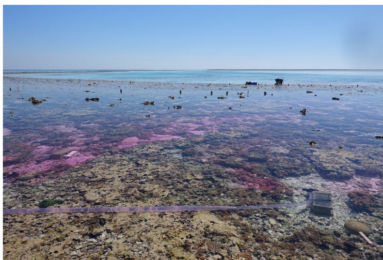
Figure 1. Rhodamine dye flowing over a coral reef flat study site during a study in One Tree Island, Australia (Albright et al., 2016). NaOH was used as an active tracer to raise alkalinity, and rhodamine was used as a passive tracer to account for mixing and dilution. Changes in the alkalinity-to-dye ratios were used to isolate the change in alkalinity flux that was associated with an increase in net community calcification on the reef flat.
