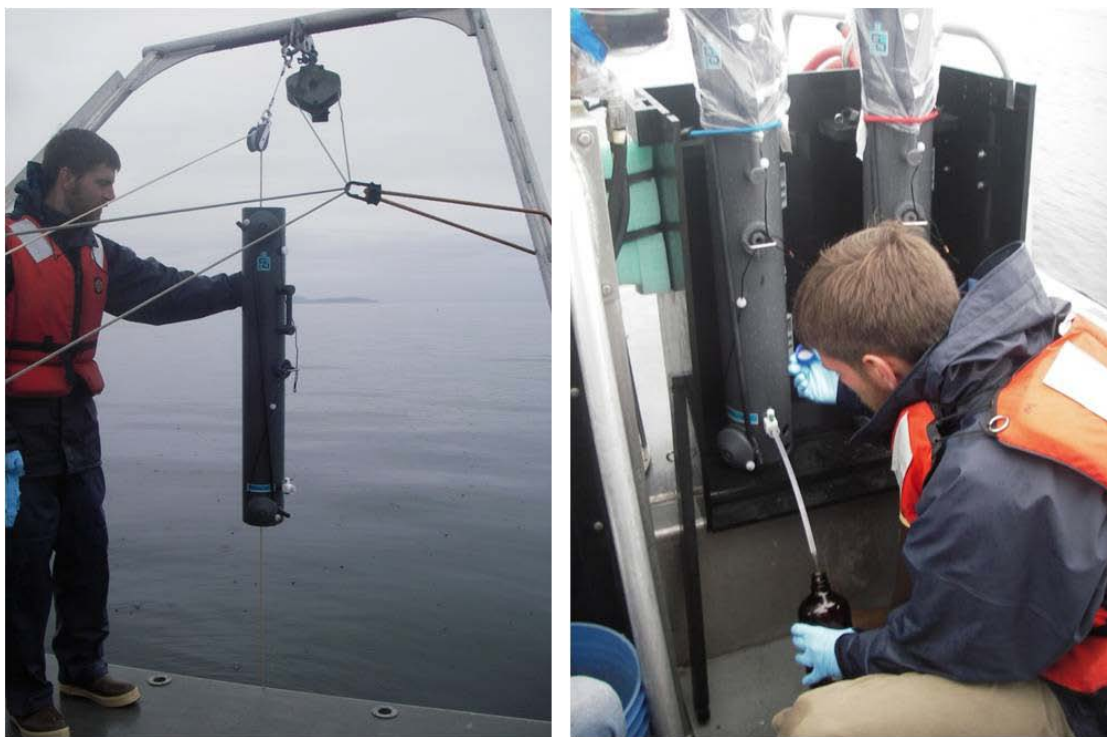
Figure 2. Collecting samples from the marine water column using GO-FLO samplers.
