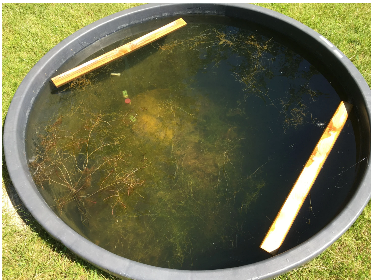
A close-up of one of the mesocosm pools, where insects and other species under study live among the plants and sediment they would in the real world to get a better understanding of how microplastics might affect them in their natural habitat. Credit: Martin Wagner
