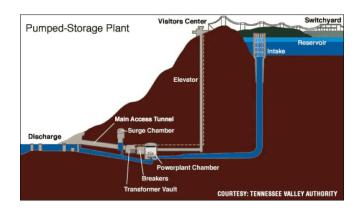
This diagram illustrates how pumped hydro storage works with an upper and lower reservoir.
