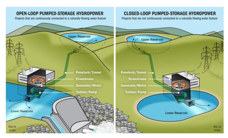
Pumped hydro projects can generally be described as "open loop" or "closed loop" systems. Courtesy of Rye Development
