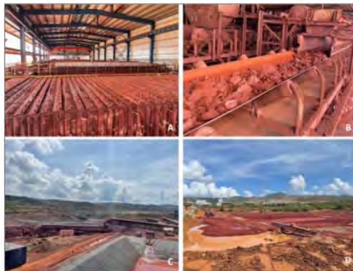
Figure 7-6: Dry stack tailings facility operation
