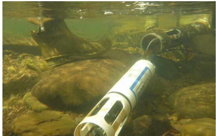
A submerged sonde, temporarily out of its protective, camouflaging PVC sleeve.
