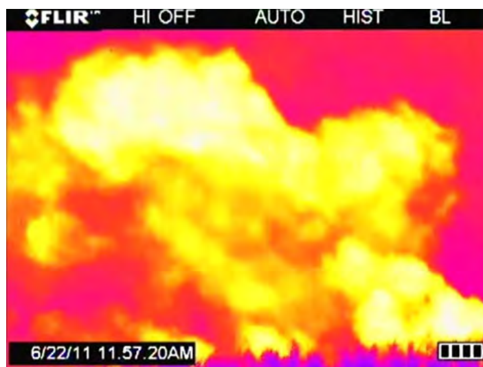
Fig. 1 Venting of natural gas into the atmosphere at the time of well completion and flowback following hydraulic fracturing of a well in Susquehanna County, PA, on June 22, 2011. Note that this gas is being vented, not flared or burned, and the color of the image is to enhance the IR image of this methane-tuned FLIR imagery. The full video of this event is available at http://www.psehealthyenergy.org/resources/view/198782 . Video provided courtesy of Frank Finan
