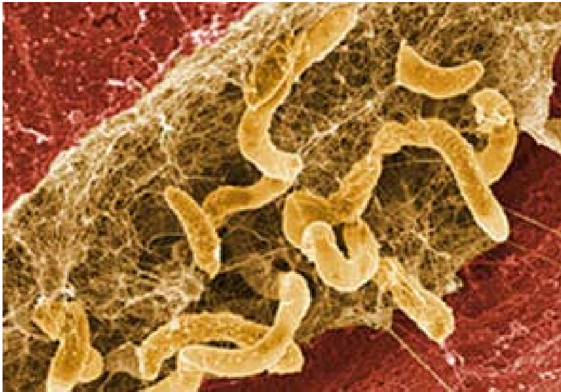
Figure 2: Biofilm of Desulfovibrio desulfuricans Growing on a Hematite Surface
