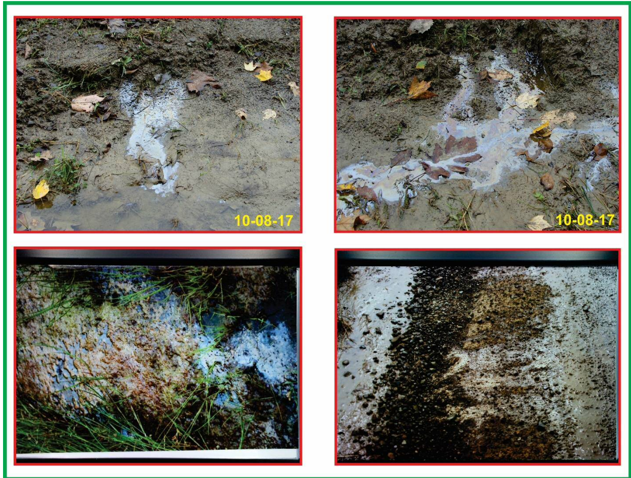
Figure 1. Sediment discoloration along Warren County, PA roadways where brine spreading has occurred. The bottom right photo shows brine flowing from a road surface into a drainage ditch.
