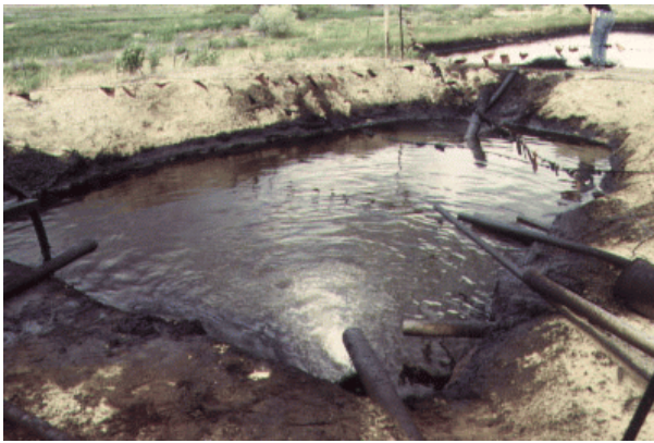
Figure A-2. Pits are commonly used in Wyoming to separate oil from produced water. Produced water from a heater treater is discharged into a pit to further separate oil from produced water prior to discharge.
