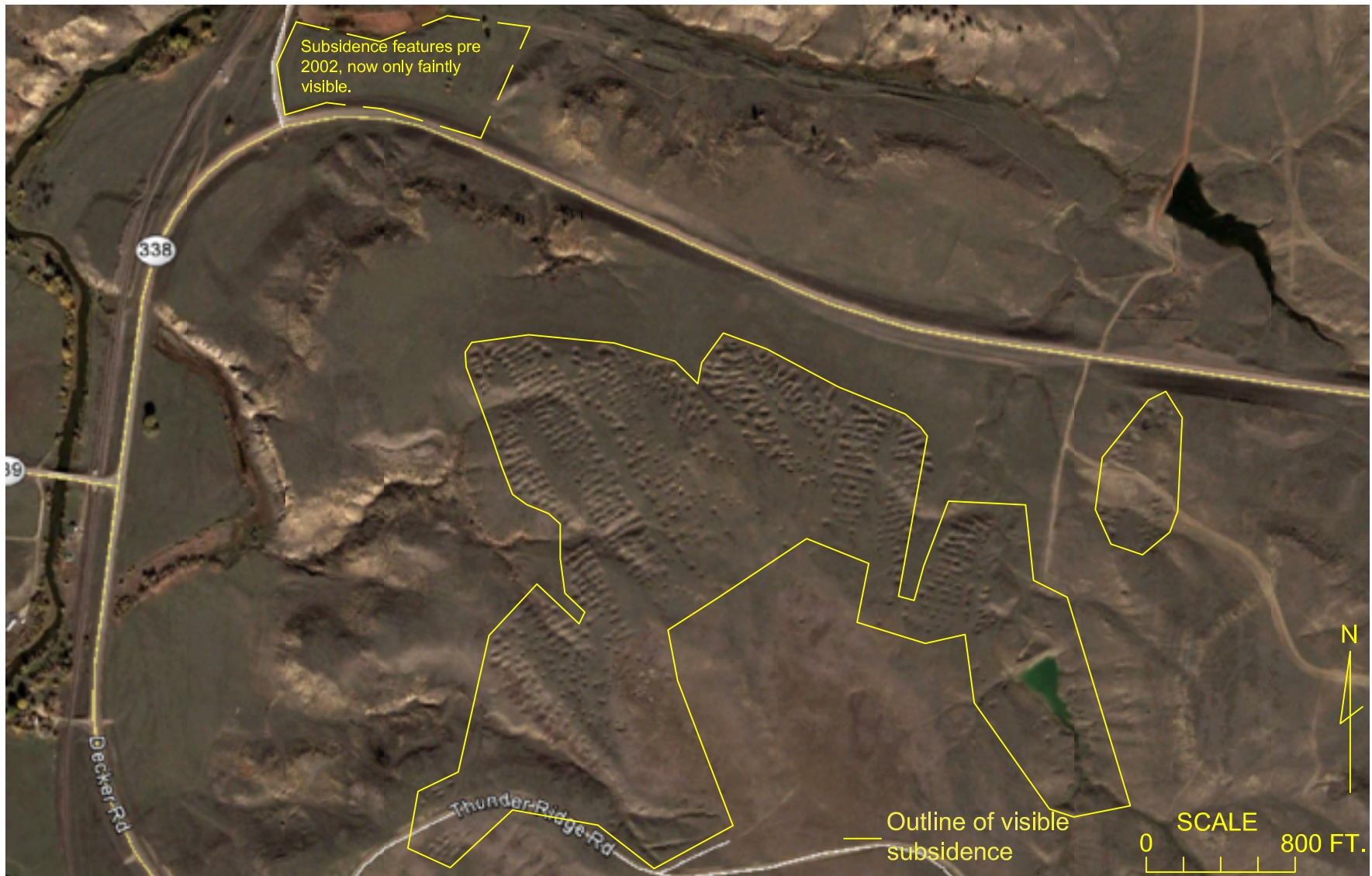
FIGURE 7.5 AREA 4 MINE SUBSIDENCE FROM UNDERGROUND MINING OF DIETZ MINES NO. 5 TO 8. IN THE DIETZ COAL SEAMS AT ROUGHLY 20 TO 150 FT. BELOW GROUND SURFACE (DUNRUD, C. R., AND OSTERWALD, F.W., 1980).
