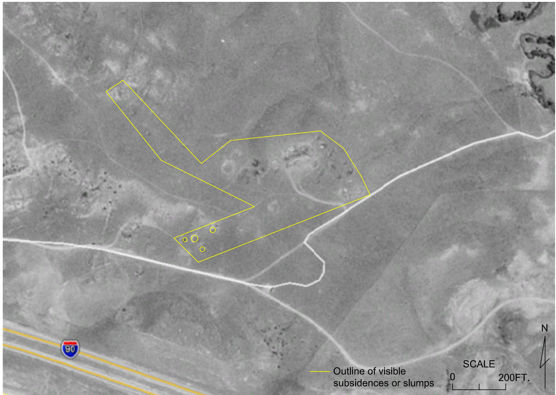
FIGURE 7.3 AREA 2 MINE SUBSIDENCE FROM UNDERGROUND MINING OF THE OLD ACME NUMBER 3 MINE IN THE UPPER CARNEY SEAM. MINE DEPTH IN THE NOTED SUBSIDENCE AREA IS 60 TO ABOUT 160 FT. (ADD_D5-4_EX_1_OVB_ISO_R1).
