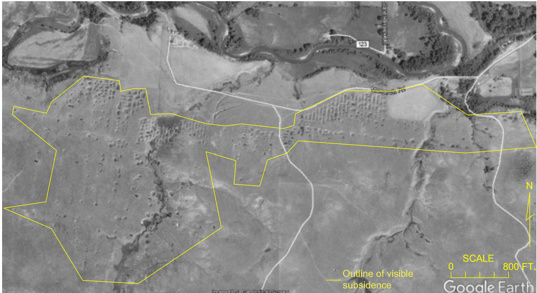
FIGURE 7.4 AREA 3 MINE SUBSIDENCE FROM UNDERGROUND MINING OF THE OLD MONARCH MINE IN THE MONARCH SEAM. MINE DEPTH IS APPROXIMATELY 35-50FT (DUNRUD, C. R., AND OSTERWALD, F.W., 1980).
