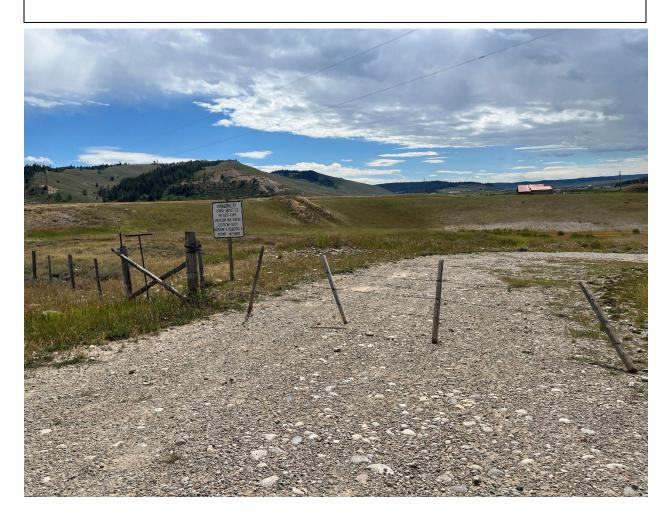
Picture of existing gravel pit taken on September 1, 2024 showing there are still large pools of standing water despite Bondurant experiencing one of the driest spring and summer on record. With normal rainfall, the size of the standing water pools would be much higher and spill over sections of the poorly maintained berms into wetlands and Dell Creek.
