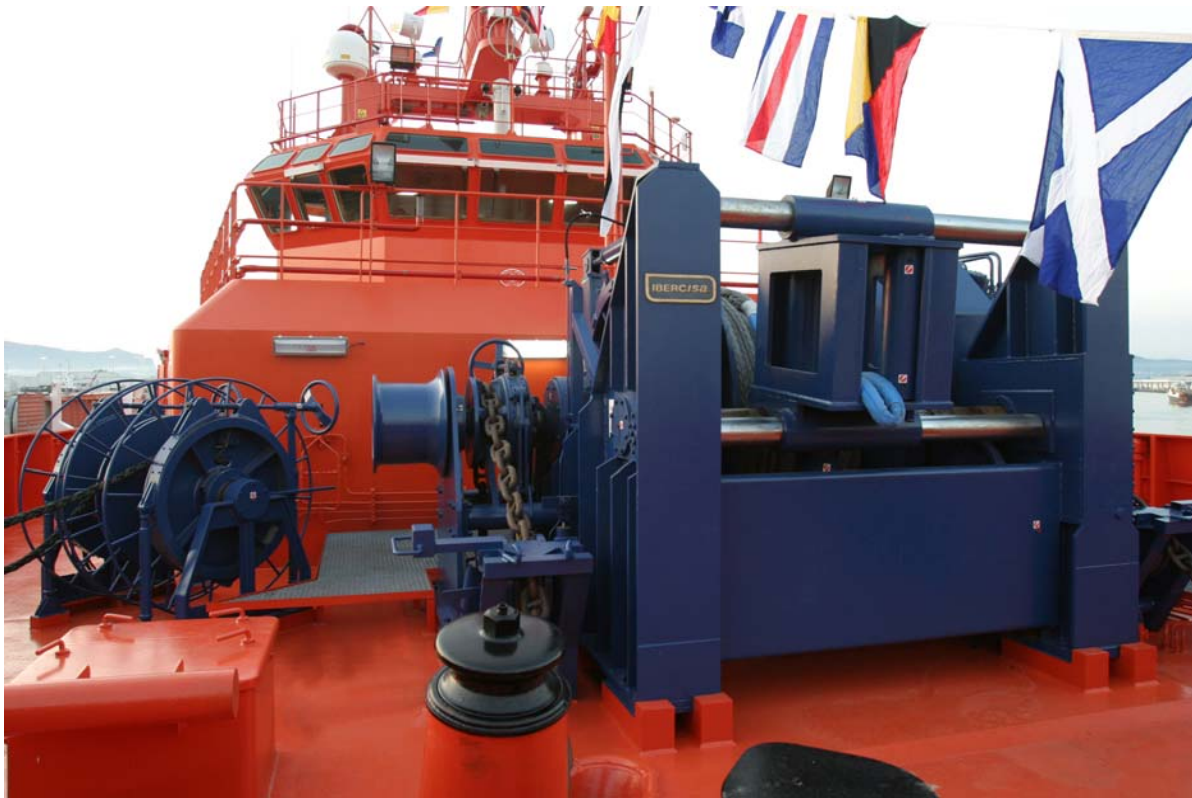
Figure 26 Combined towing winch and anchor windlass installed on the bow of Luz de Mar , taken from Reference 46
