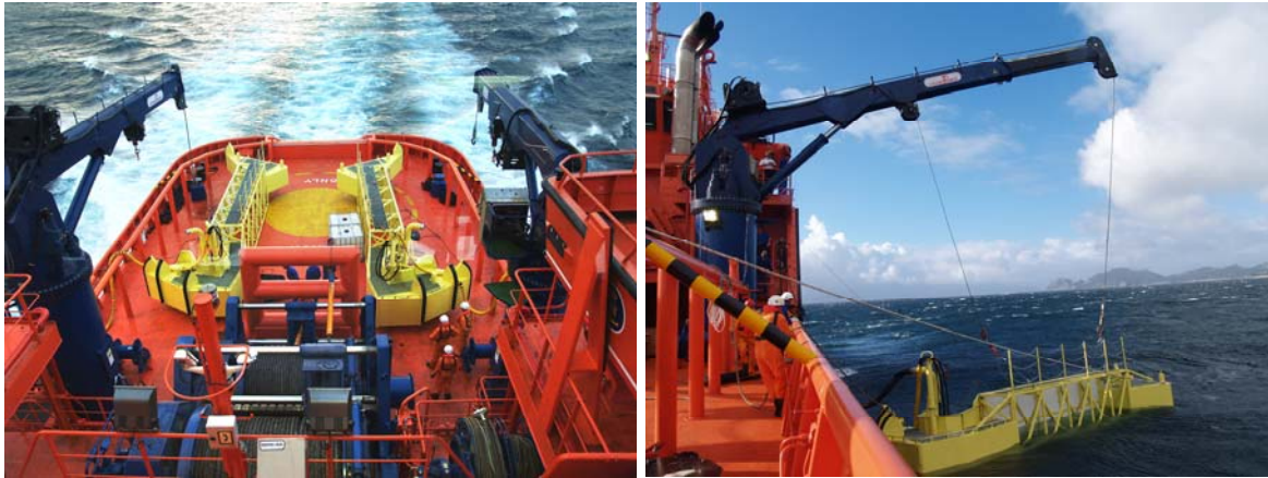
Figure 21 Deployable skimming arms on Luz de Mar , used for oil spill recovery (Reference 39)
