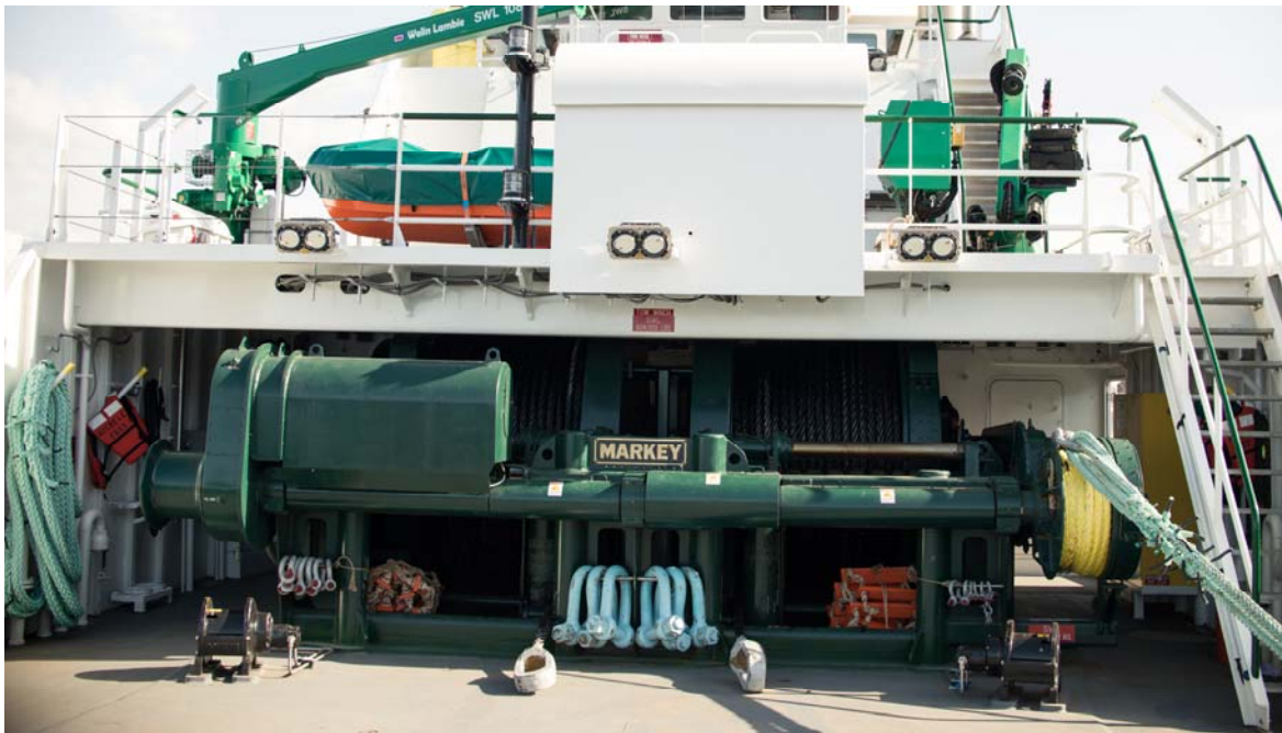
Figure 3 Photo of the same winch shown in Figure 2, outfitted and installed on an oceangoing tug; photo courtesy of Markey Machinery
