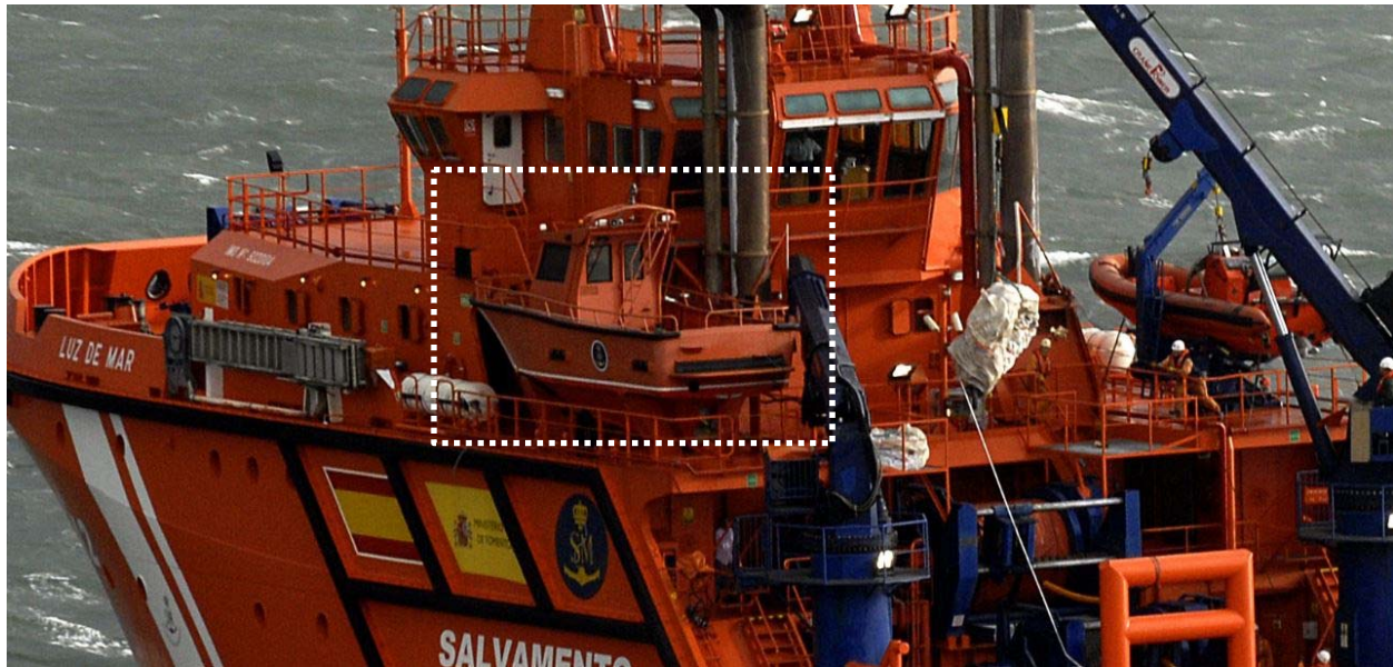
Figure 19 9.9m aluminum workboat in its stowed position on the port side; SOLAS compliant fast rescue boat also visible on the starboard side; photo courtesy of https://twitter.com/salvamentogob
