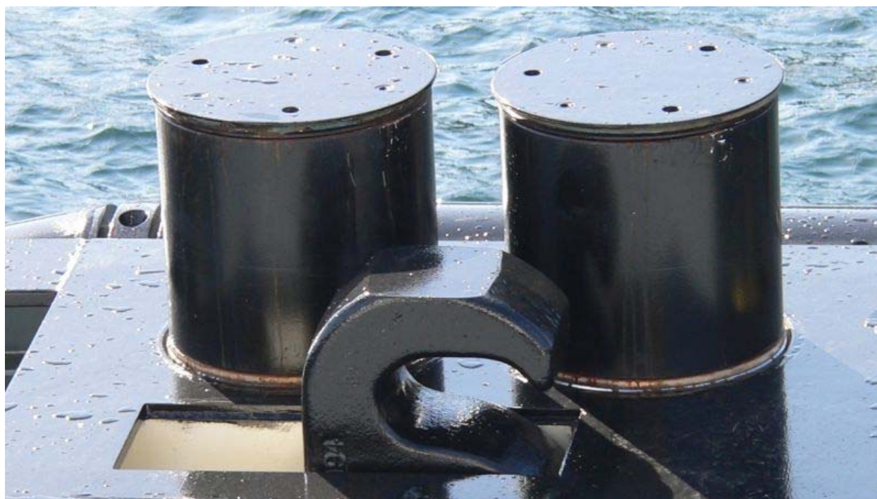
Figure 4 Photo of the conventional Smith Berger tow pin and hook assembly installed on the current SERVS escort tugs, accessed from https://maritime-executive.com/corporate/tow-pins on 3/20/2021
