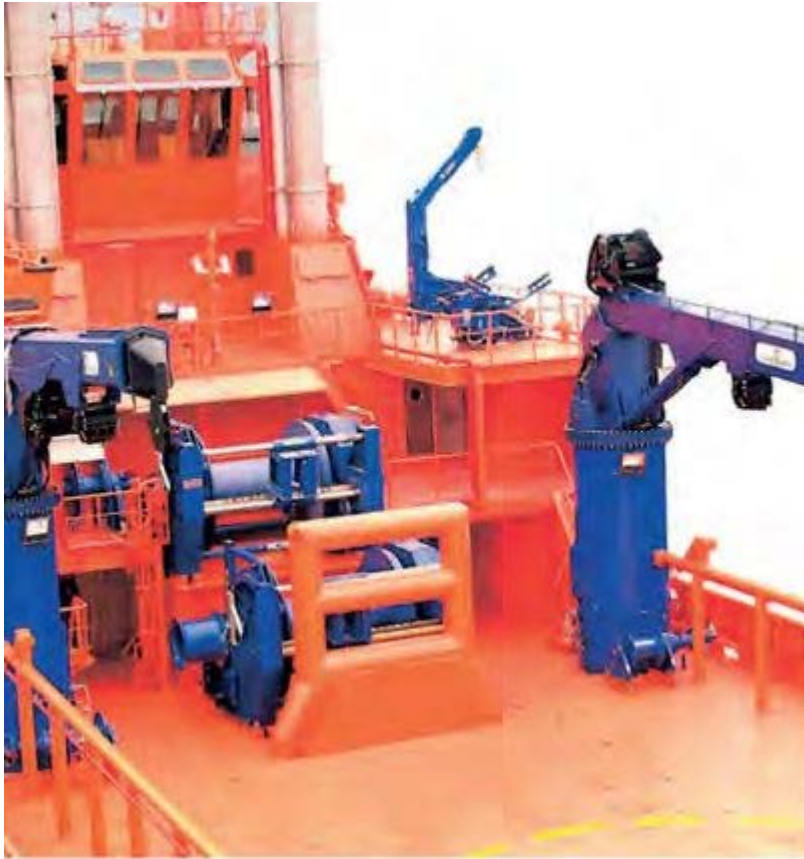
Figure 25 Aft towing winches on Luz de Mar prior to installation of the tow wire, taken from Reference 45
