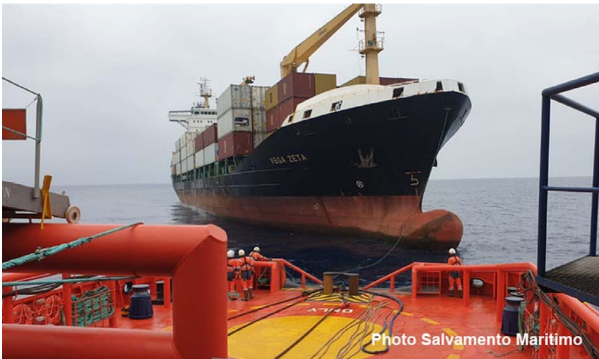
Figure 16 Stern gate or “breakwater” on Luz de Mar in the down position while taking a disabled vessel in tow, accessed from https://www.fleetmon.com/maritime-news/2020/29453/disabled-container-ship-towed-valencia/ on 3/22/21
