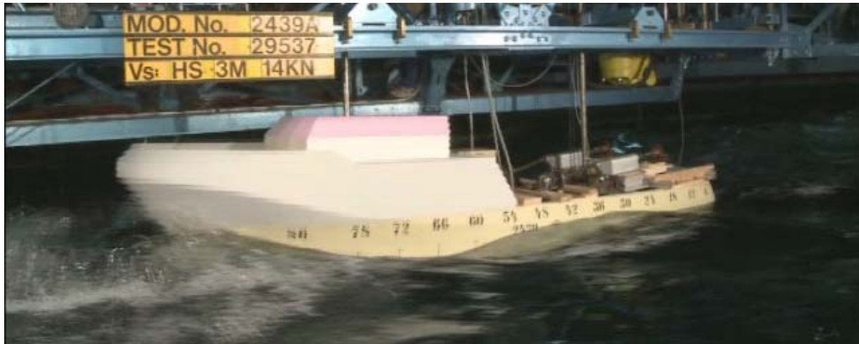
Figure 9 Photo of the RAsalvor 6000 series hull form undergoing model testing; photo courtesy of RAL, 3/30/2021
