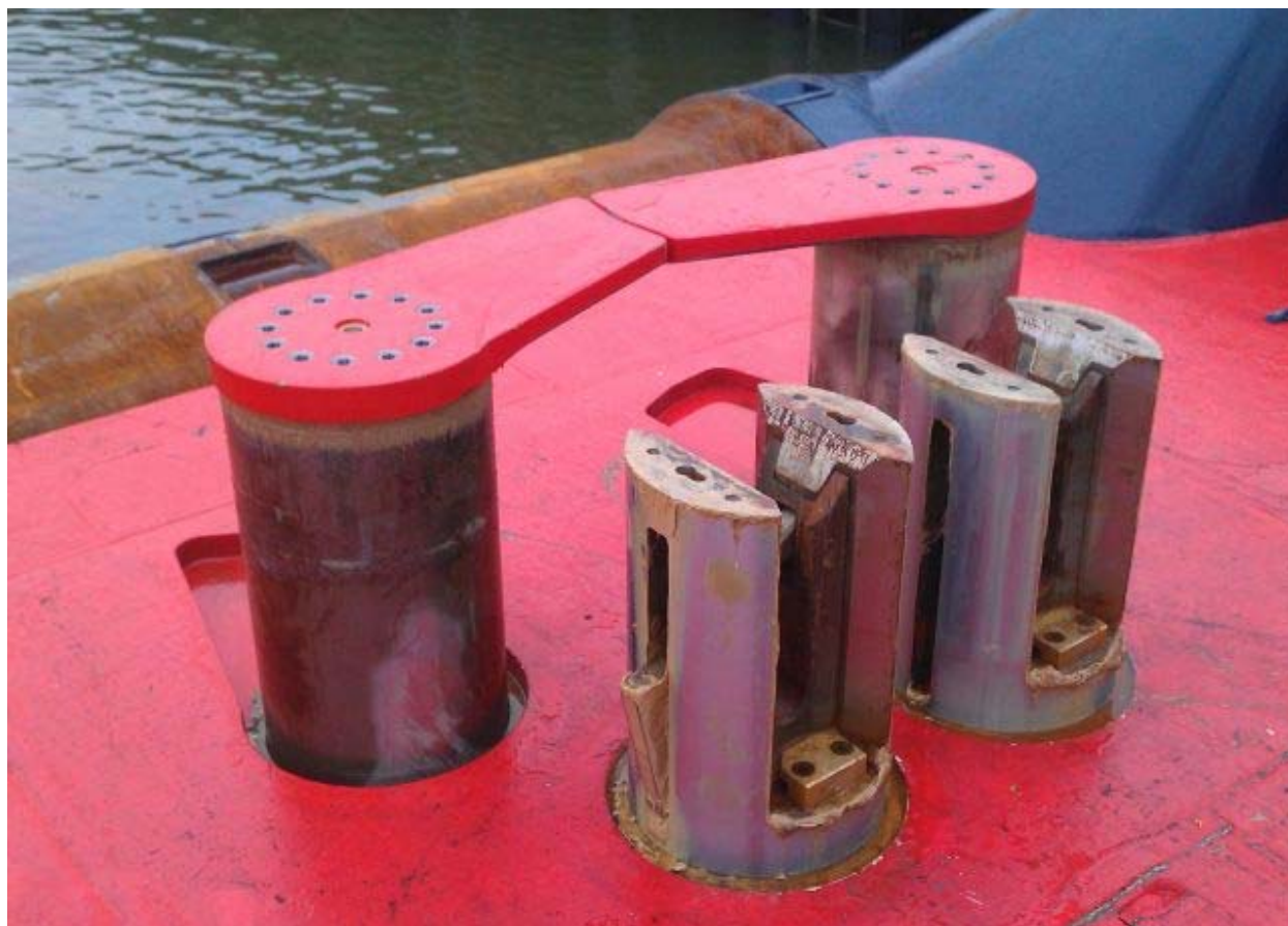
Figure 5 “Top locking” type tow pins with Karm forks, accessed from https://www.maritimejournal.com/news101/onboard-systems/deck-equipment-and-lifting-gear/second-generation-towing-pins-popular on 3/20/2021
