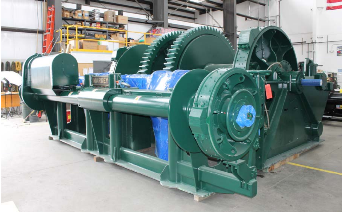
Figure 2 Example of a side-by-side double drum ocean towing winch, configured for underwater wire deployment; photo courtesy of Markey Machinery
