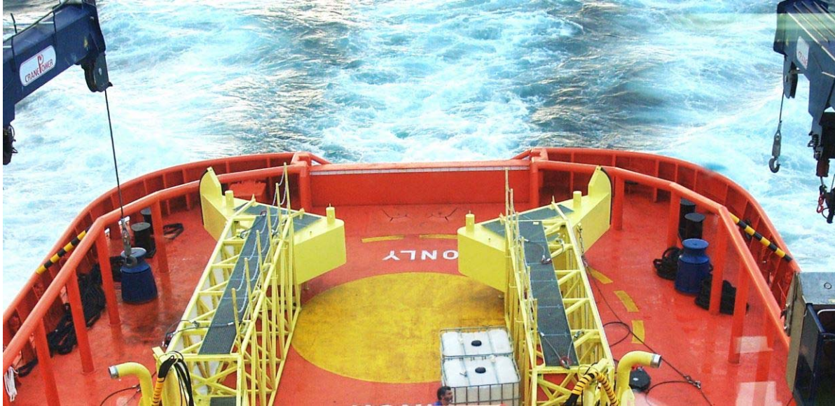
Figure 15 Stern gate or “breakwater” on Luz de Mar in the up position (Reference 39)
