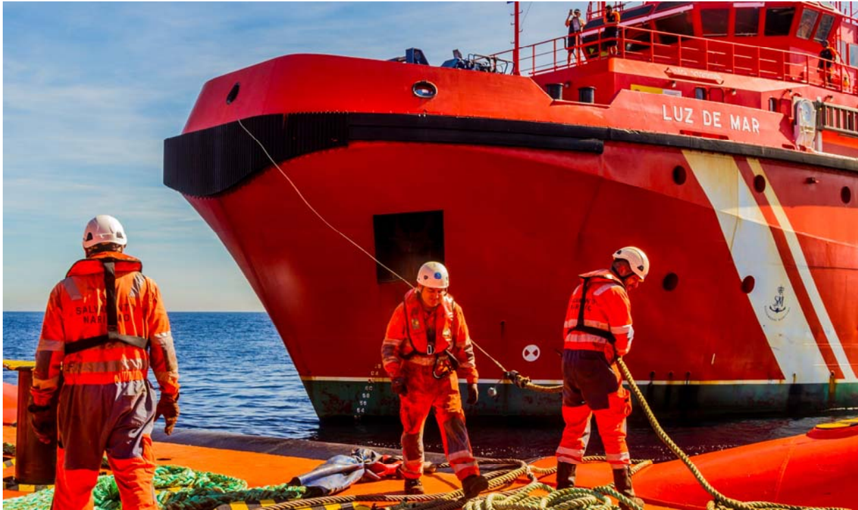
Figure 27 Bow form and fendering on Luz de Mar , accessed from https://balearicyachtshow.org/2020/stand/100/salvamento-maritimo on 3/29/2021
