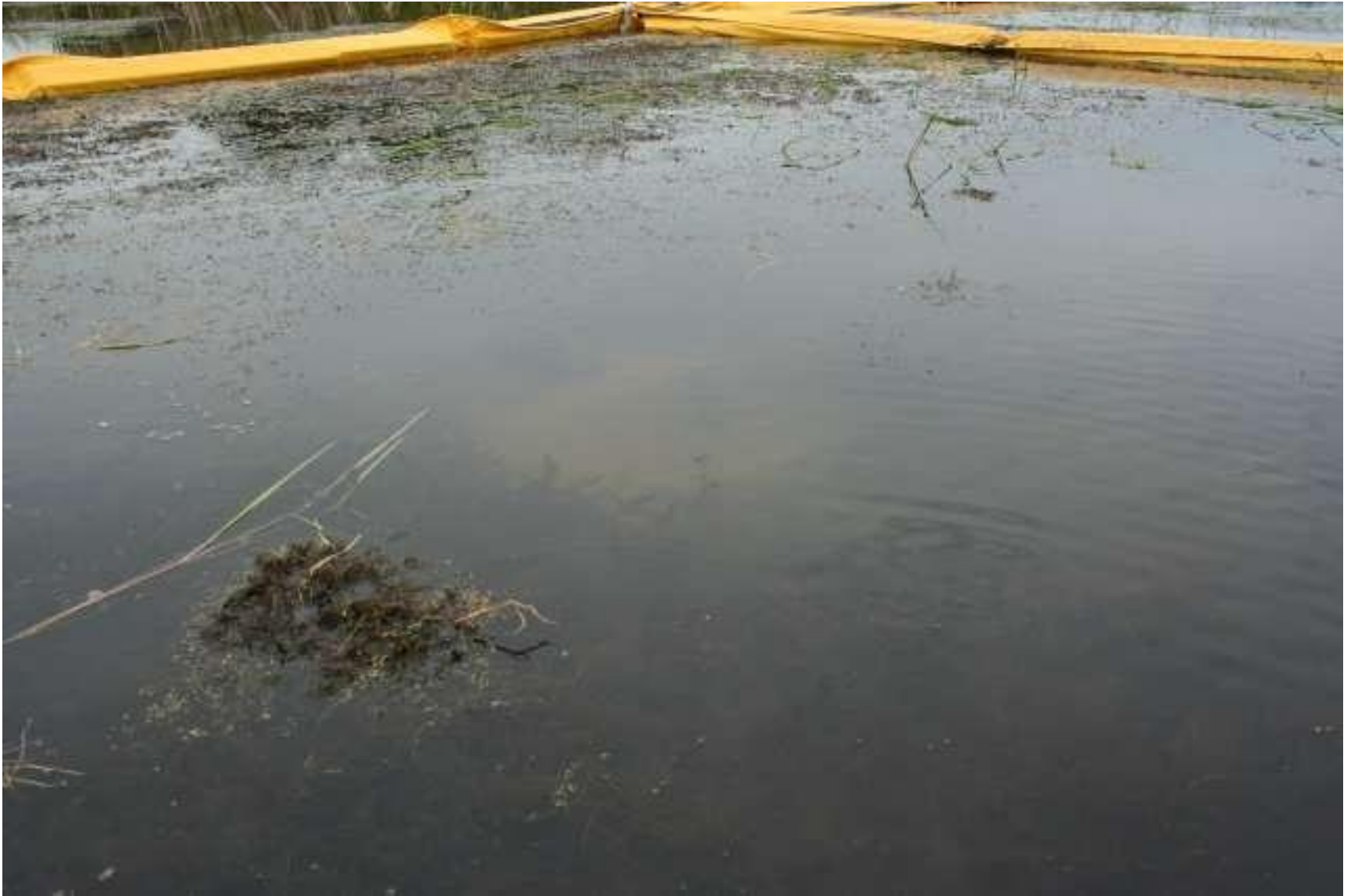
Turbidity indication of frac disturbance near frac mound at Hay Creek.
