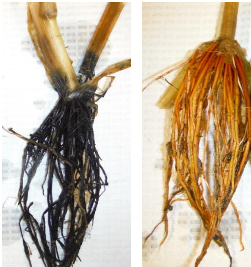
Figure 1. Sulfate-amended root (left) and control root (right). Sulfate-amended root has black color extending from about 0.5 cm above the root ball down to the tips of the roots (not shown). Control root has amber color characteristic of iron (hydr)oxides, especially 2-3 cm below root ball.
