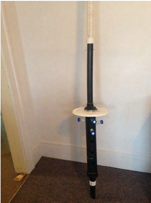
Figure 24. Peeper sediment pore water sampling device
