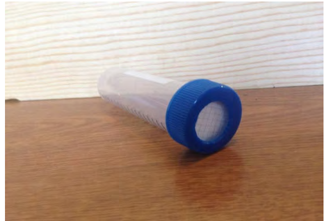
Figure 25. Example of a 50-mL centrifuge tube used for peeper sediment pore water quality measurements
