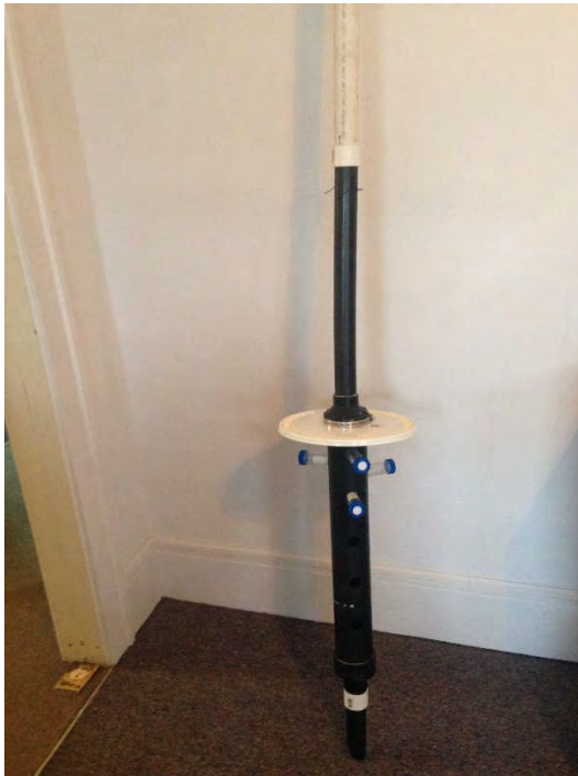
Figure 24. Peeper sediment pore water sampling device
