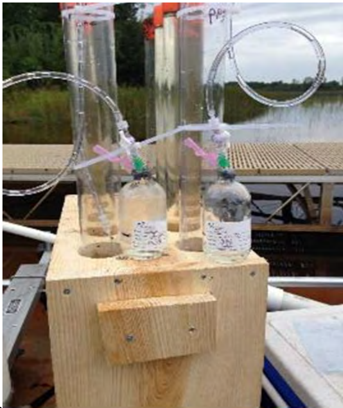
FIGURE 34. RHIZON FILTER APPARATUS IN USE FOR SAMPLING SEDIMENT PORE WATER
