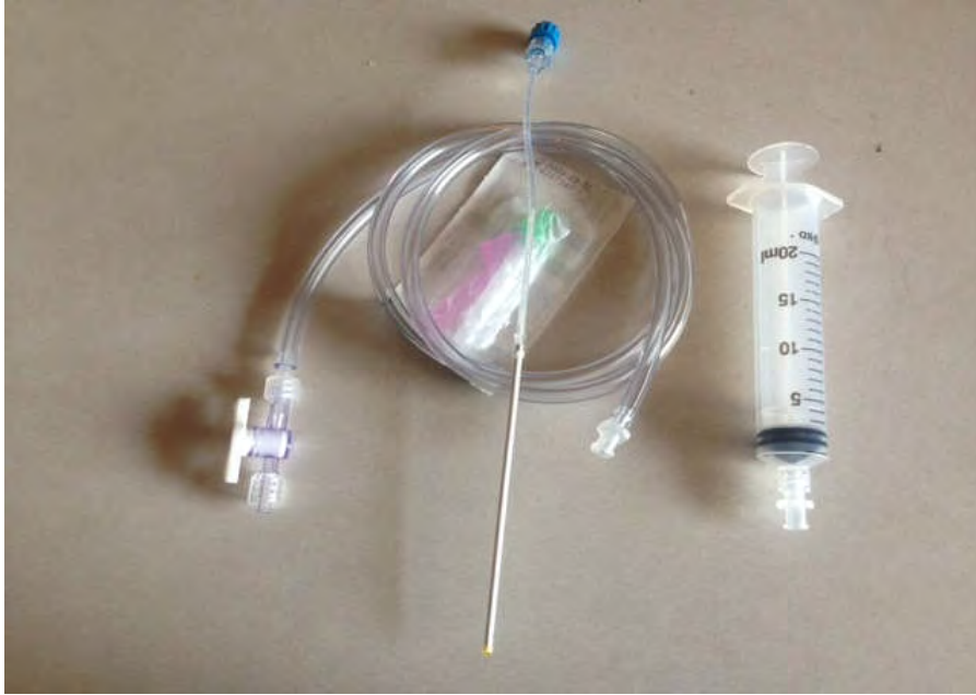
FIGURE 33. RHIZON FILTER APPARATUS USED FOR SEDIMENT PORE WATER SAMPLING. NOT PICTURED – 125-ML EVACUATED GLASS SAMPLE CONTAINER
