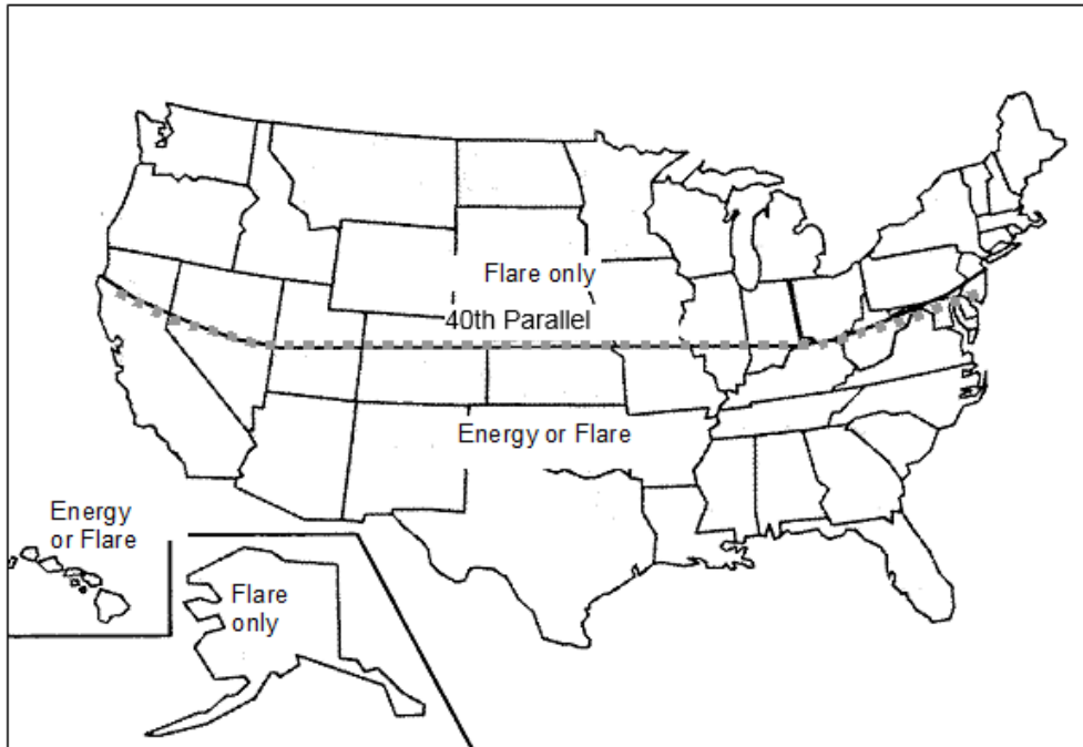
Figure 3. Covered lagoons - locations suitable for biogas to energy conversion generally fall below the 40th parallel.
