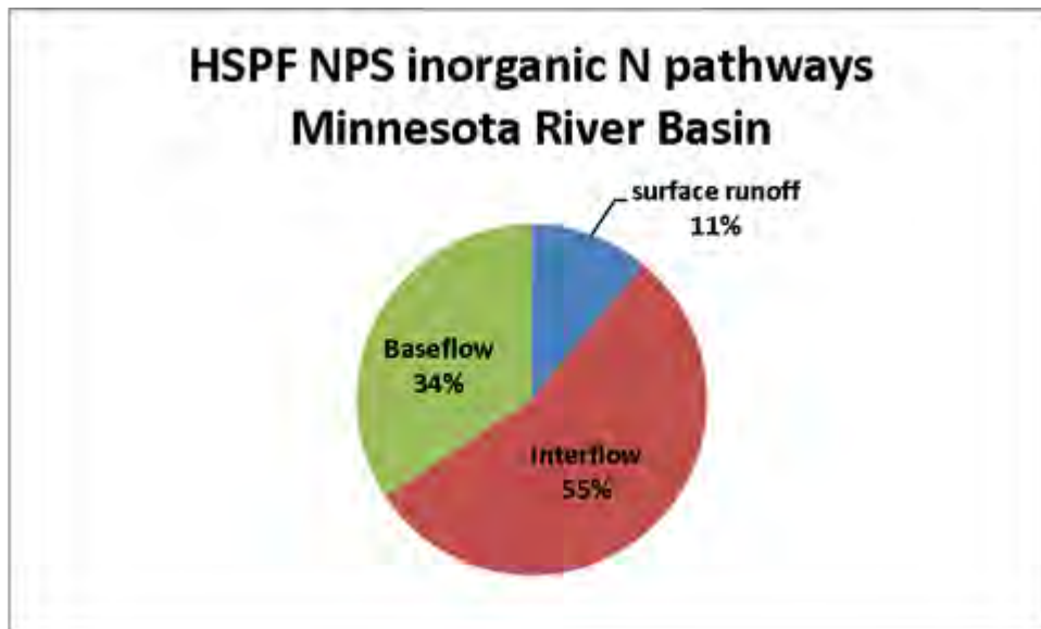
Figure 7. HSPF model estimates of the proportion of nonpoint source inorganic N which enters surface water through the three model flow pathways in the Minnesota River Basin during a typical precipitation year within the timeframe 1993-2006.
