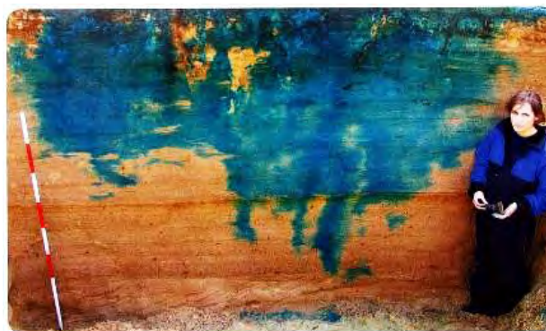
Figure 1. This photograph shows the cross section of a soil profile with blue dye poured at the soil surface. The wetting front and irregular preferential flow pattern are clearly shown as the blue dye percolates through the soil. This can help explain why soil water nitrate concentrations from one lysimeter can have markedly different concentrations when compared to another lysimeter only a few feet away. Figure adapted from Haarder et al, 2011.
