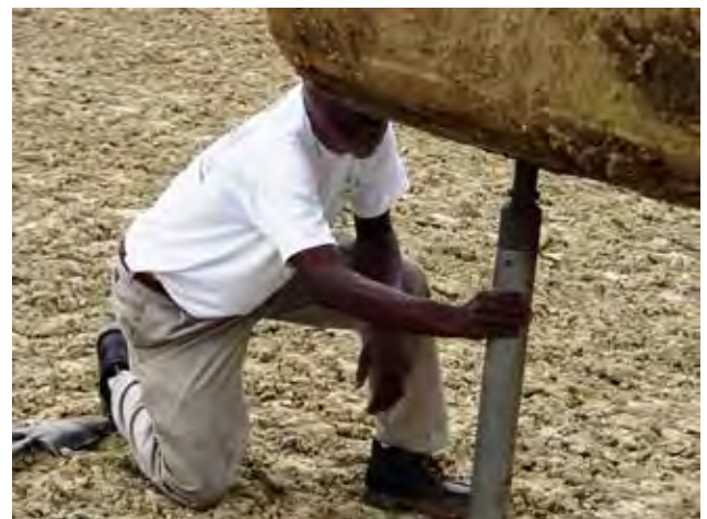
Figure 10D–32 Shelby tube sample being obtained with backhoe bucket used to force tube into clay liner (Photo credit Jody Kraenzel, NRCS, NE)
