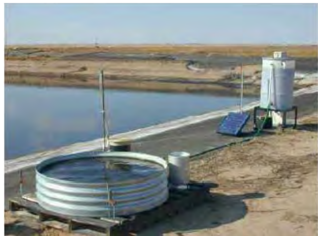
Figure 10D-34 Equipment used to monitor evaporation at an agriculture waste storage lagoon. Measurements are used in total lagoon seepage evaluations.
