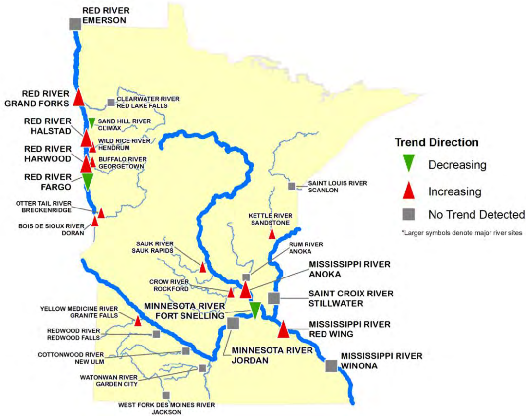
Figure 3. River monitoring site locations at sites with enough information to determine mid-range (20-year) flow-adjusted nitrate concentration trends. QWTREND was used to assess trends at these sites, except that the flow-adjusted bootstrapped Seasonal Kendall test was used at tributaries to the Minnesota River, the Sauk River and Kettle River.
