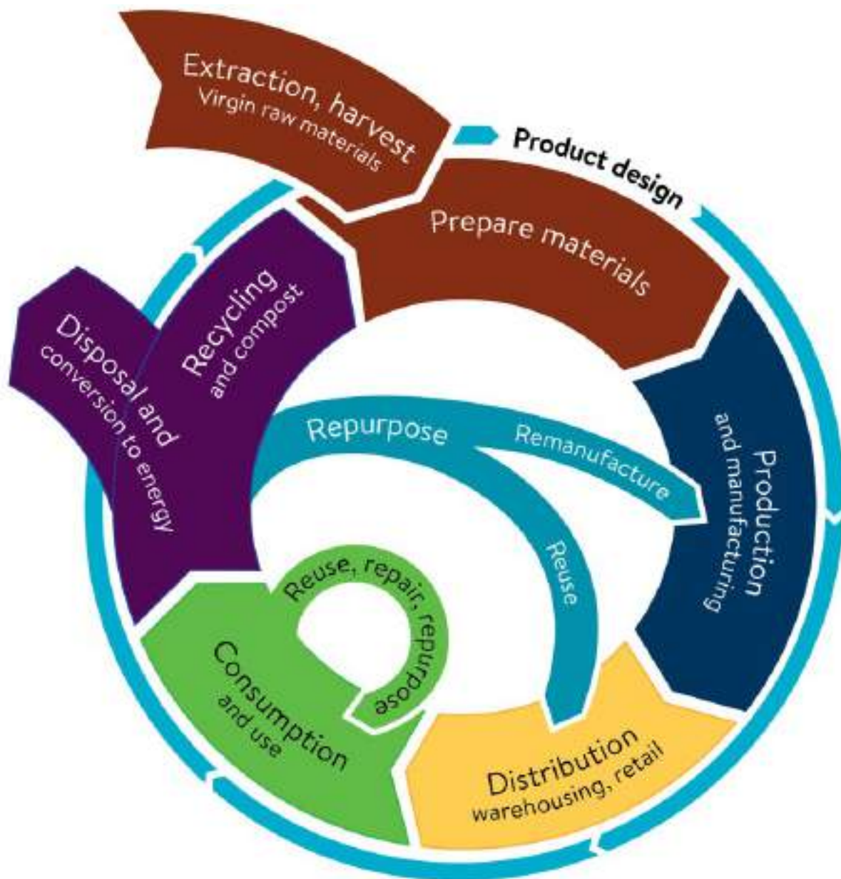
Figure 5. LCA: a methodology for modeling the environmental impacts of a material or product from raw material extraction through end-of-life management
