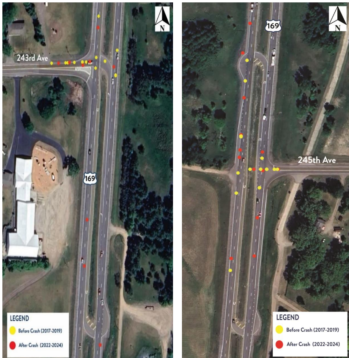
Exhibit 2-10. Before-After Crashes at J-Turn Intersections
