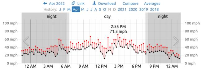
Measured wind speed at approximately **10 meters** above an open field (black dots). Civil twilight and night are indicated by shaded overlays.
