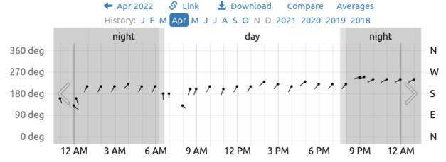
Measured wind direction at approximately 10 meters above an open field (black dots). Civil twilight and
