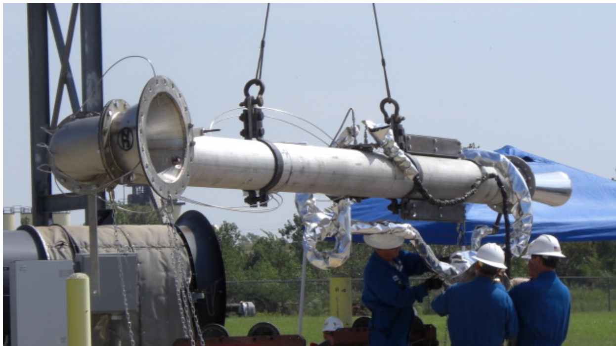
Figure 4-8. Sample Collector at Near Ground Level. Collector inlet is at foreground and eductor is at far end. In photo, Zink personnel make adjustments to heated transfer line supports. Shackles and cable at center allow crane to lift and position Sample Collector.
