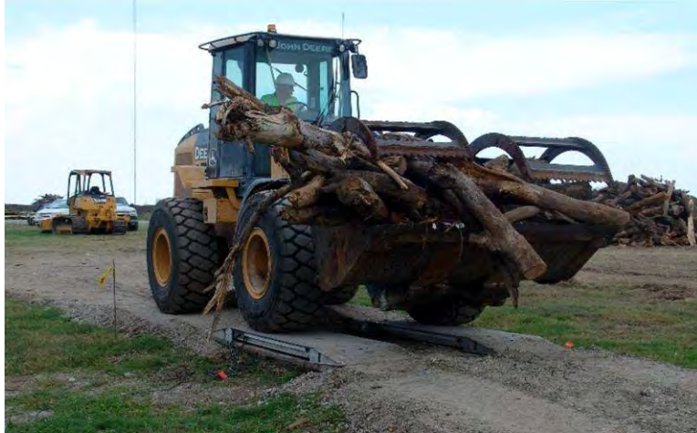
Figure 4-3. Loaded Front Axle Being Weighed
