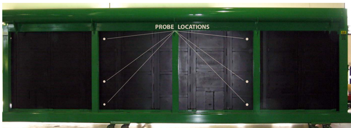
Figure 4-14. Location of Thermocouple Probes on ACB Walls
